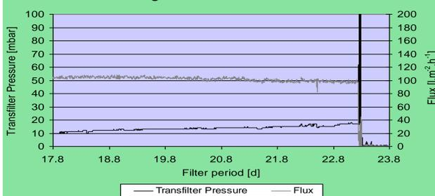
Figure: Example of the general behavior of the mesh filter in the start up phase. Data: Flux 100 L/[m<sup>2</sup>.h], MLSS 3.5 g/L, and the blocking effect
