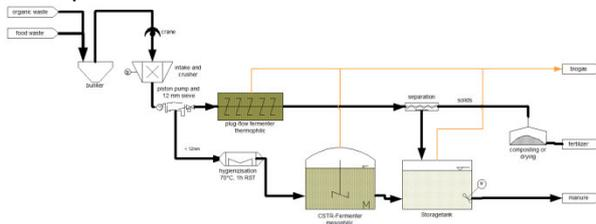
In a general attempt to **keep the system as simple as possible** we favour one stage systems without hydrolysis, but instead design the system in a straight forward approach with as little moving parts as possible.
