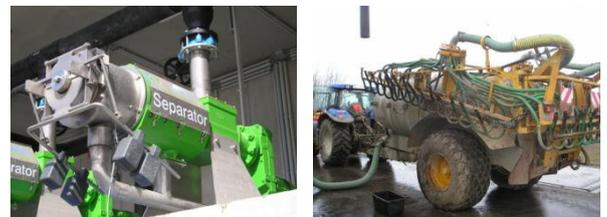
Since the output of the plug flow fermenter is too wet to be handled effectively it needs to be separated prior to any further composting or drying.
