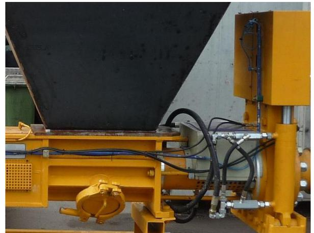
After this step the material is pressed with a piston pump through a special screening unit to remove all physical contaminants larger than 12 mm, such as metals, ceramics and plastics.
