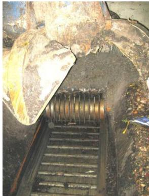
The level of contamination of the feedstock material is one of the key considerations. It usually has significant levels of contaminants such as plastic, glass or metals and they have to be removed prior to entering the digesters.
